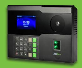
P serial is a multi-biometric identification time & attendance and access control terminal, which can connect with third party electric lock, door sensor, and exit button etc.
